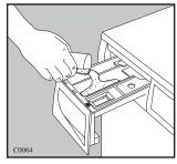
If required, pour fabric softener into the compartment marked \& (the amount used must not exceed the "MAX" mark in the drawer). Close the drawer gently.
